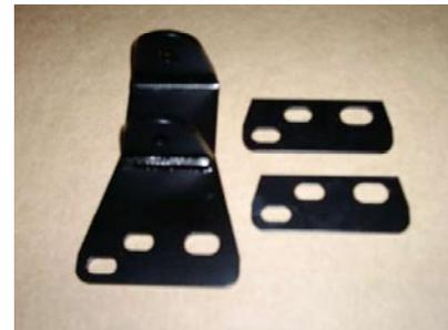
BETWEEN BRACKET AND CROSS MEMBER(the spacers used are determined by the amount the body overhangs the rear crossmember which is unique to individual vehicles, it maybe necessary to use the 2mm spacer 4mm spacer or both for the bracket to be level with the body) USING THE 3 M10 BOLTS NUTS & WASHERS SUPPLIED.
